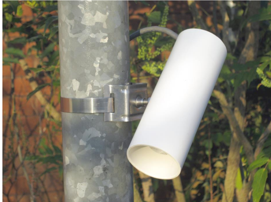
Figure 4. An IR-SS fitted to a pole with an optional band clamp fitting
